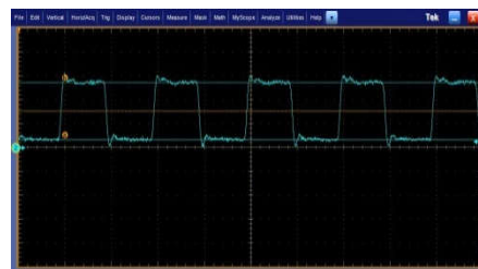
Digital Modulation at 10 MHz for square signal input
