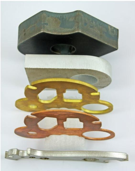
Cutting samples of the BIMO-FSC with machine controlled adjustment of focus position and diameter; provided by MicroStep: 6 mm stainless steel, 1.5 mm copper, 3 mm brass, 15 mm aluminum, 25 mm mild steel (bottom to top).
